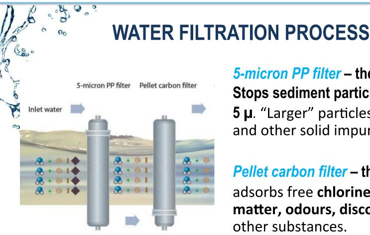
5-micron PP filter – the 1st barrier. Stops sediment particles size up to 5 μ. "Larger" particles as rust, sand, and other solid impurities.
